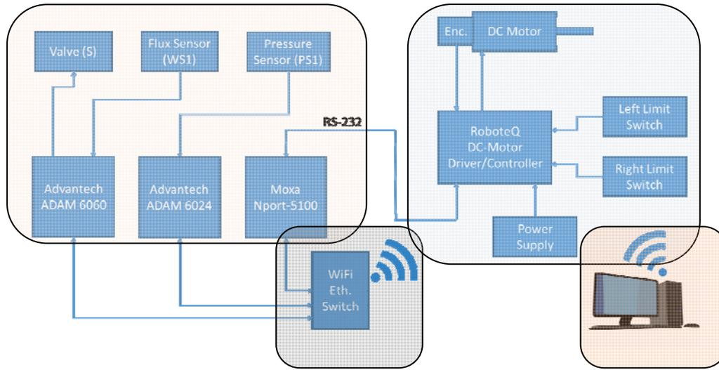
Figure 2: Block diagram of the electronic control system.
