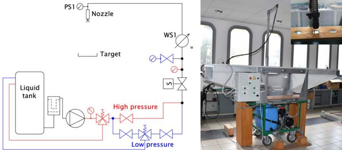
Figure 1: Block diagram of the hydraulic components (PS1: pressure sensor; WS1: water flux sensor; S: solenoid valve); on the right a picture of the test bench with a particular of the acquisition system.
