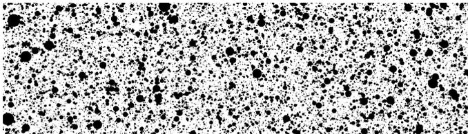
Figure 3: Example of image of water sensitive paper simulated.
