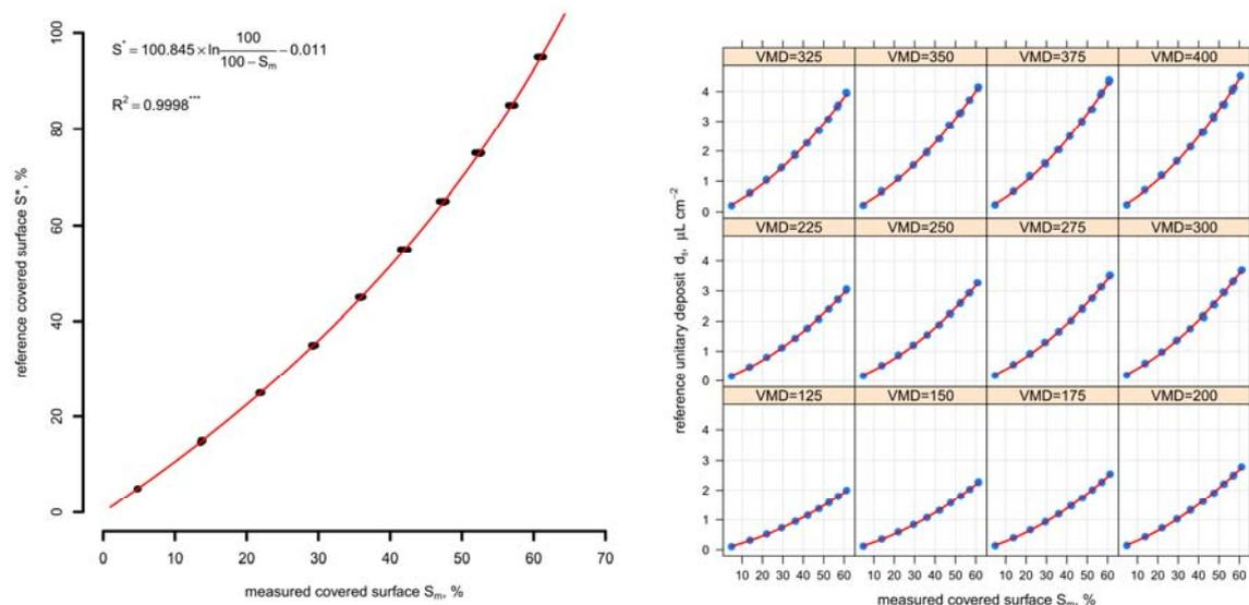
Figure 4: Correlation between measured ( $S_m$ ) and reference ( $S^*$ ) percentage of covered surface.
