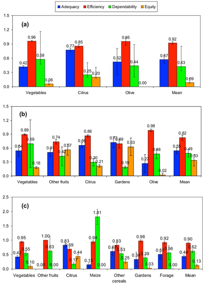
Figure 2 – Current indicators (means and std. devs.) of adequacy (“AD”), efficiency (“EF”), dependability (“DE”) and equity (“EQ”) in the water delivery systems “Angitola 3DMF” (a), “Angitola 6DMF” (b) and “Savuto” (c).
