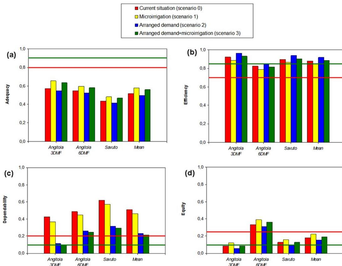
Figure 3 – Indicators of adequacy (a), efficiency (b), dependability (c) and equity (d) in the water delivery systems "Angitola 3DMF", "Angitola 6DMF" and "Savuto" under the current and the three simulated scenarios (the red and green lines show the limits "poor" and "good" respectively).
