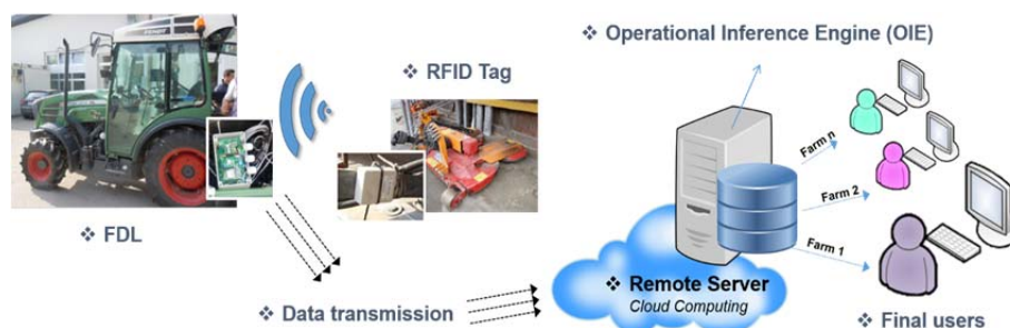
Figure 2. In the figure the conceptual model followed is reported. The operational parameters were collected and transmitted to a remote sever (left part of the picture), here a specific operational inference engine interprets the raw data and translates them into intelligible information in order to be consulted by the farmer.
