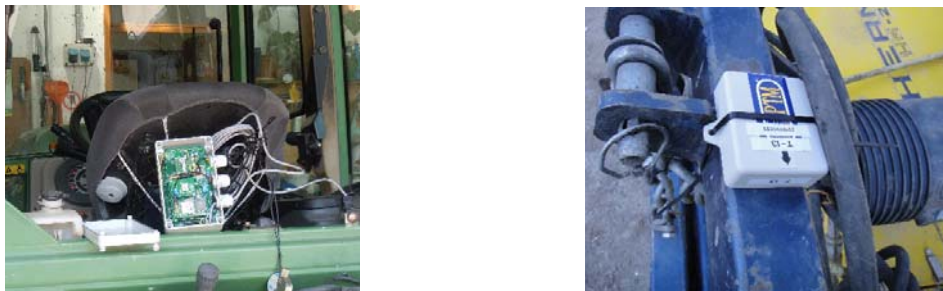
Figure 1: The left figure shows the FDL installed on the tractor. Thanks to its simply design configuration, the power supply is taken from the cigar lighter, while the right figure shows active RFID fixed at the frame of a mulching machine.
