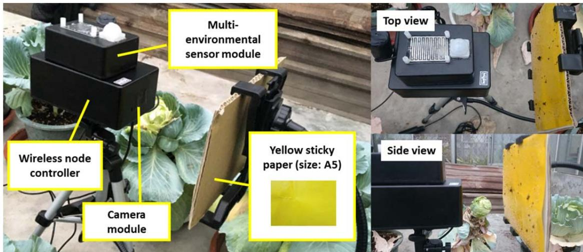
Figure 1: Wireless imaging and sensor node (top view and side view) with part labels
