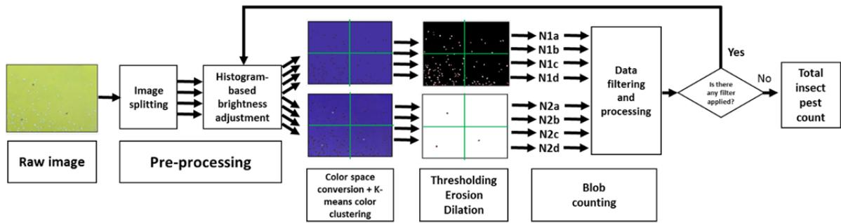
Figure 4: Insect pest counting image and data processing algorithm flowchart
