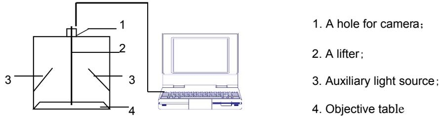
Figure 1 Experiment box for taking pictures
