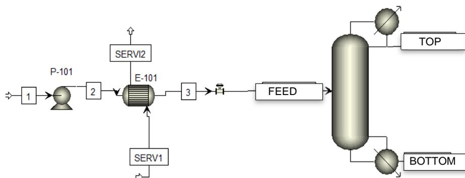
Figure 2: Configuration of Reactive Distillation
