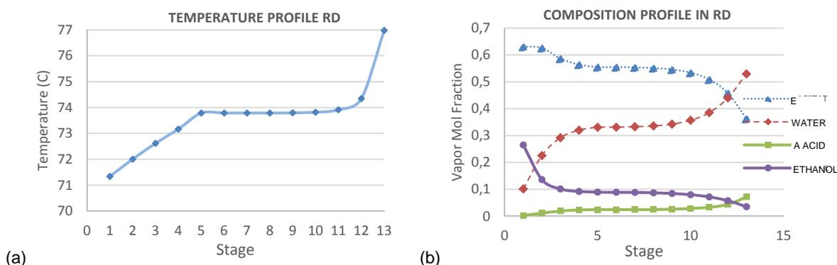
Figure 3: (a) Temperature profile of RD, (b) Composition profile in the RD
