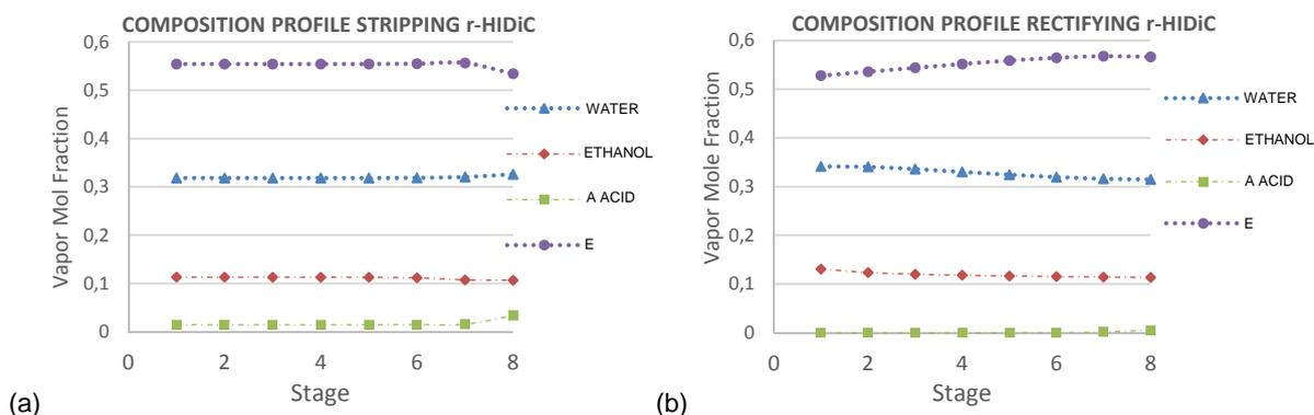
Figure 4: Composition profile in the r-HiDiC column, (a) Stripping Section, (b) Rectifying Section
