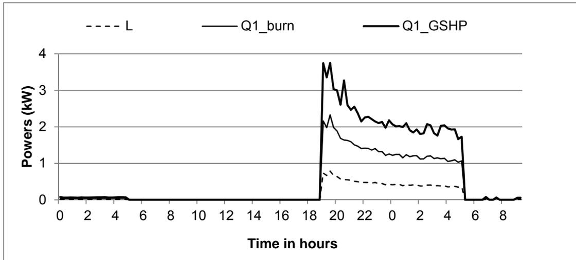
Figure 4: Fuel cell electric power, ground source heat pump and hydrogen burner heating powers.
