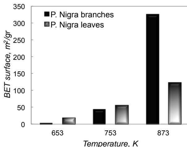
Figure 3: BET surface of char obtained from pyrolysis of branches and leaves at different temperatures.
