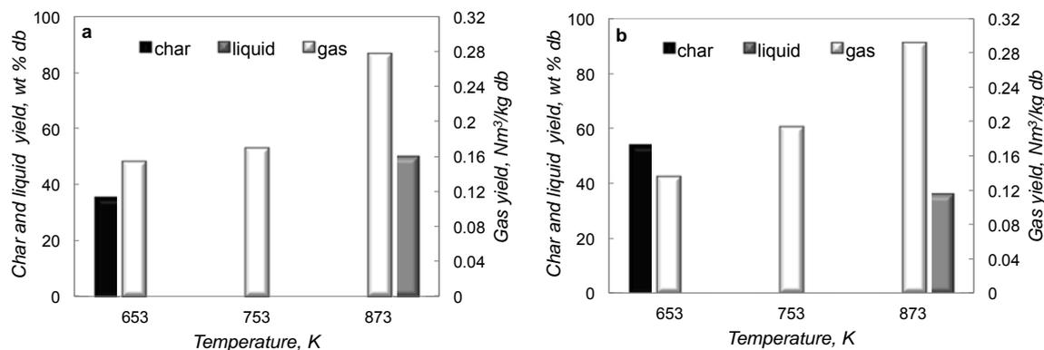
Figure 1: Products yield obtained at different pyrolysis temperature from branches (a) and leaves (b).
