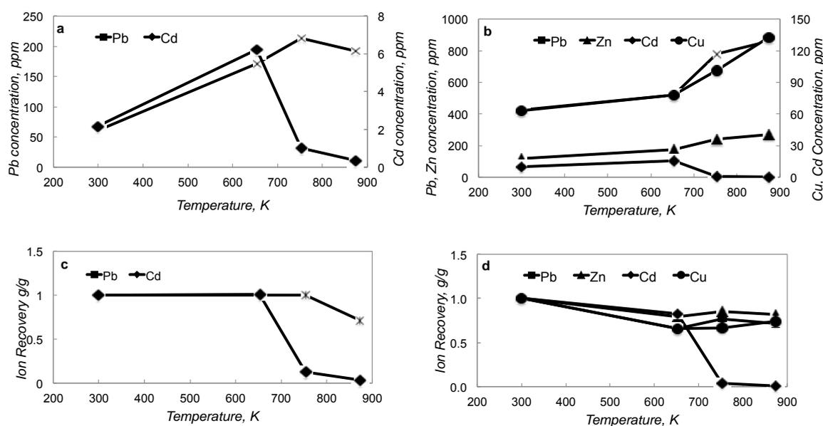
Figure 2: Concentration and Ion Recovery of PTEs in the chars from branches (a and c, respectively) and leaves (b and d, respectively).
