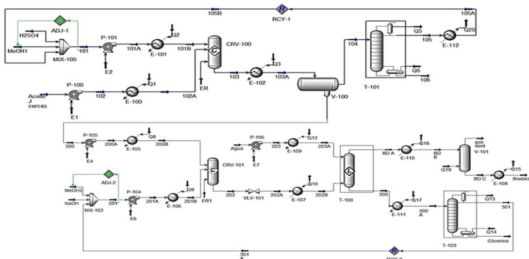
Figure 1: Simulation stage of obtaining biodiesel
