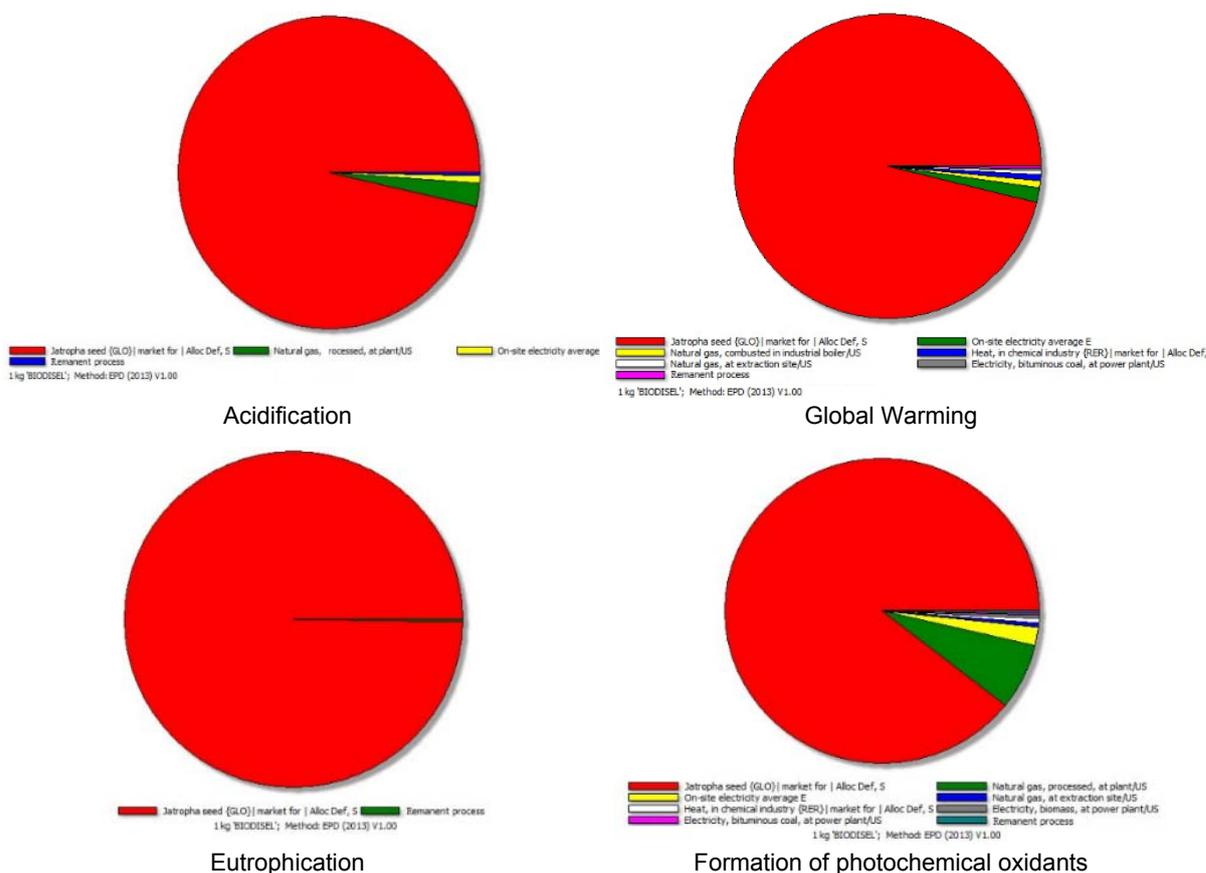
Figure 2: Life cycle impact assessment results of 1 kg of biodiesel of *Jatropha Curcas*
