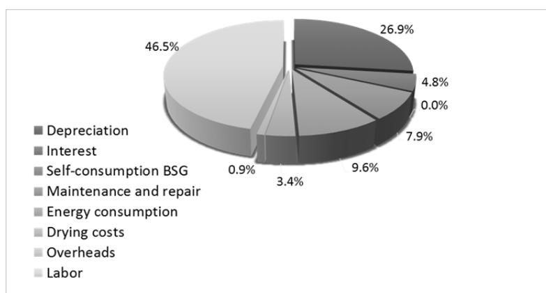
Figure 1: Percentage breakdown of annual operating costs of the small plant of pellets production in relation to  $1,600 \text{ h y}^{-1}$  of usage
