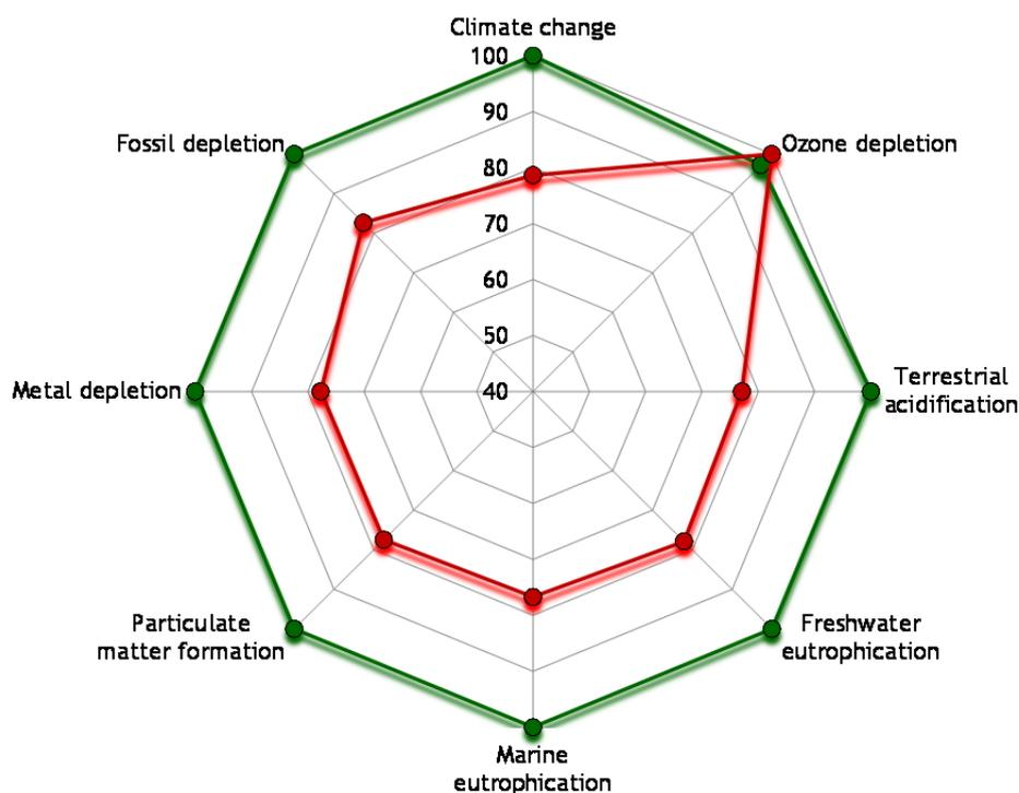
Figure 2: Relative comparison between the biodiesel produced from: flax (green) and camelina (red)
