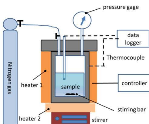
Figure 2: Hot-compressed water treatment apparatus.
