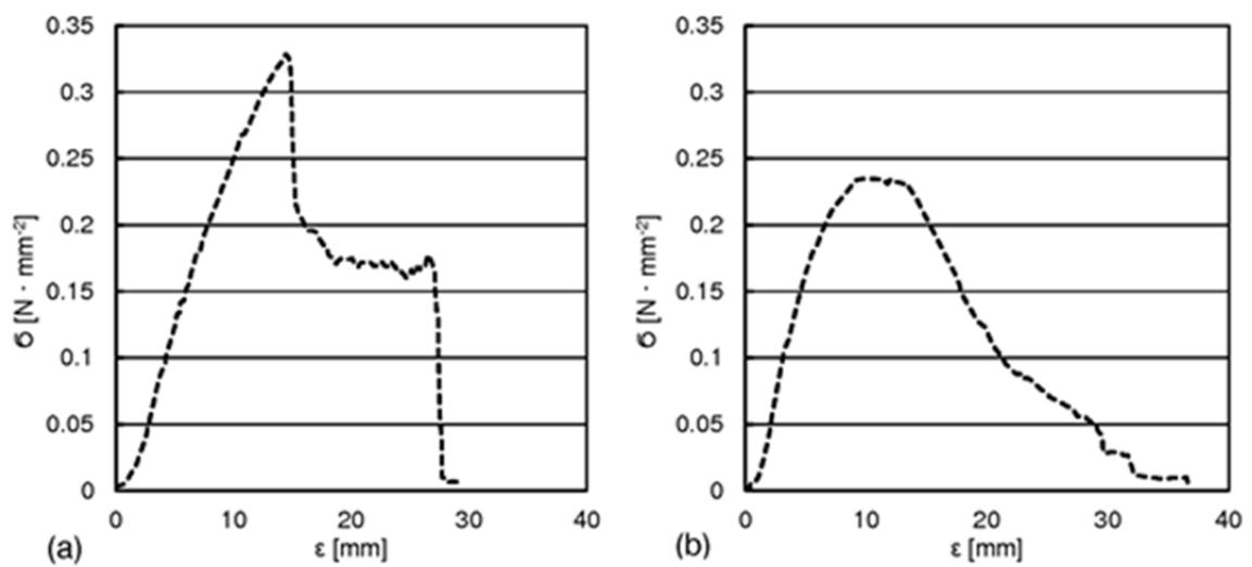
Figure 6: Three point bending loading test: I) higher initial peak, more resilient, "brittle" failure; II) lower initial peak, "ductile" failure
