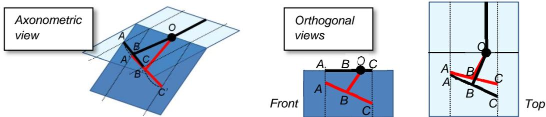
Figure 3: when an articulated vehicle is astride the edge (O: articulation joint), the front half/axle (ABC) has a double inclination (on the horiz. plane, to turn, and also due to the slope change); the dangerousness of this situation (A'B'C') is the impossibility for some vehicles to fully comply with the inclined plane, and hence the loss of contact of the wheel in C (C'); thick black/red lines: vehicle frame in the horizontal/inclined plane.
