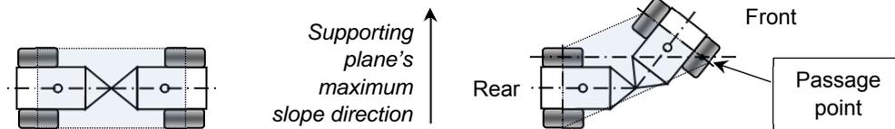
Figure 1: static stability test configurations actually forecasted for articulated farm tractors placed on a tilting plane with the support polygons evidenced; (left) straight-travelling configuration, (right) turning configuration with one of the internal wheel's axis passing through the centre of the external wheel of the part upward (UNI ISO 2012; UNI EN 2015); in this latter case the support polygon is highly distorted.
