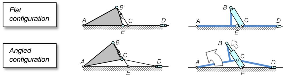
Figure 6: kinematic scheme (left) and mechanism for generating the angulation of the support plane (right); the frame of reference is fixed to the tiltable plan that is part of the facility (so it is a local frame of reference).
