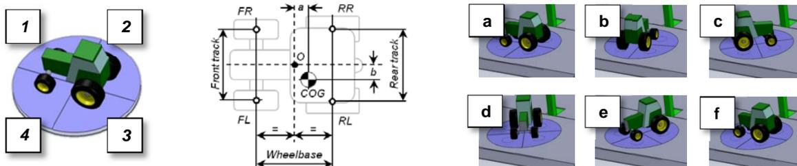
Figure 5: turntable predisposed with strain-gauges to measure the weight on each individual support (quadrant) at different inclination angles (left); the different weights ( $W_1-W_4$ ) measured by the turntable’s strain gauges are useful to localize the COG (distances  $a, b$ ) with respect to the geometric centre  $O$  of the vehicle’s support polygon (centre); measuring session for the global static stability test (pictures a-f; right).
