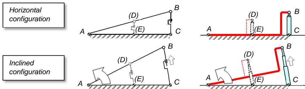
Figure 4: kinematic reference scheme and mechanism for generating the inclination of the support plane. The frame of reference is fixed to the ground on which the tiltable plan (i.e. the whole facility) is placed.
