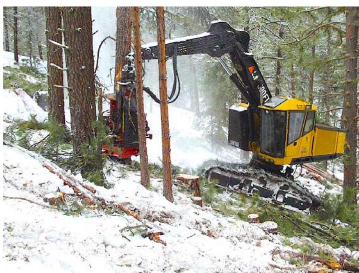
*Figure 1A & 1B: Two types of logging systems in the intermountain region of Montana and Idaho, USA. 1A) Sawyer using traditional chainsaw logging, which is used in steep mountainous conditions. 1B) Mechanical harvesting system with feller buncher common in many areas of the intermountain region.*
