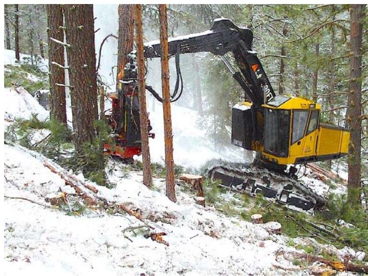
*Figure 1A & 1B: Two types of logging systems in the intermountain region of Montana and Idaho, USA. 1A) Sawyer using traditional chainsaw logging, which is used in steep mountainous conditions. 1B) Mechanical harvesting system with feller buncher common in many areas of the intermountain region.*
