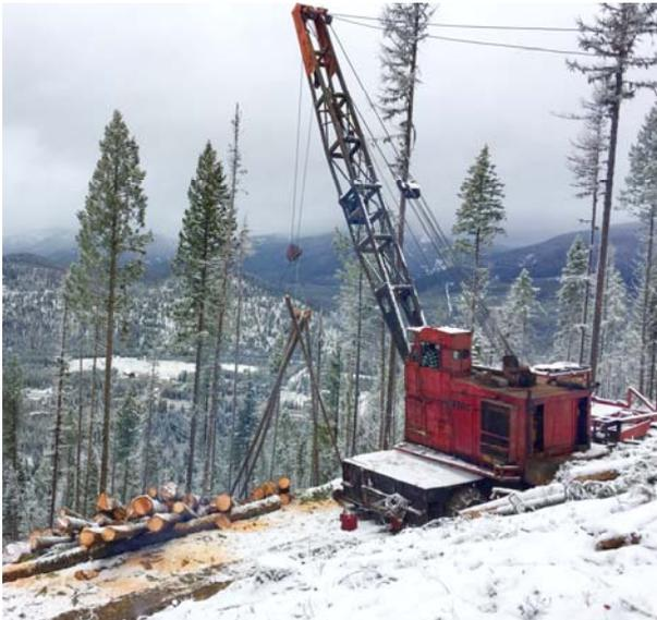
*Figure 3: An equipment operator sitting in a yarder which uses a system of cables (skyline) to pull logs from the stump up to the landing situated 300 meters in elevation above.*
