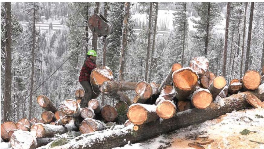
*Figure 2: Professional logger (hooker) releasing cables around logs from skyline skidding in the mountainous region in Montana, U.S. Note the proximity of the carriage overhead with the worker on the log pile.*
