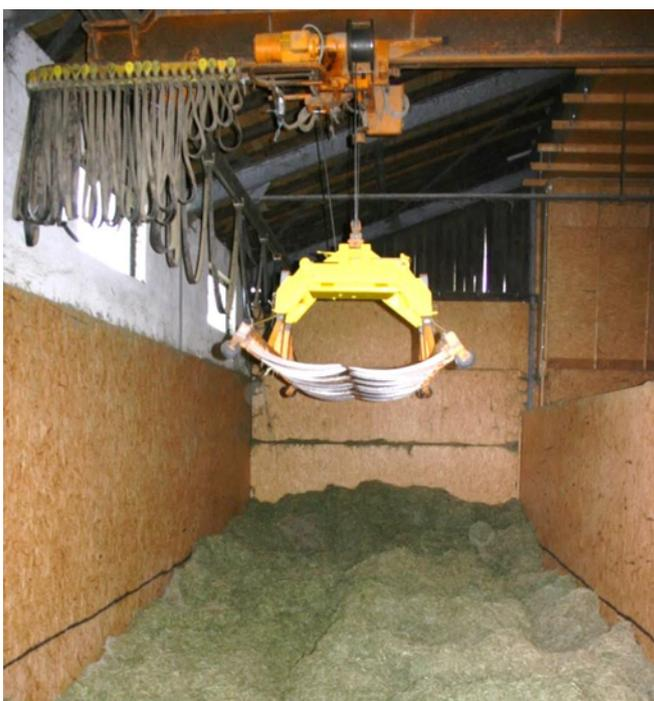
*Figure 1: Hay winch crane with remote control in park position over the drying boxes*
