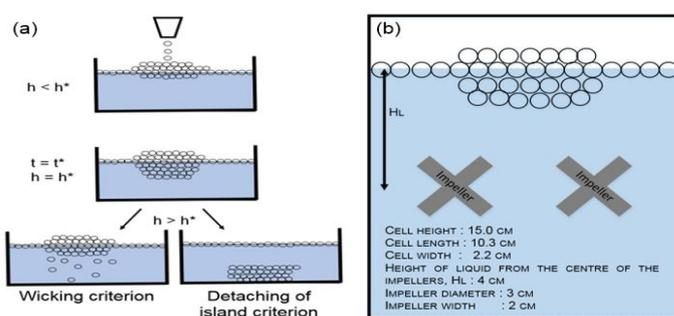
Figure 1: Experimental setup to investigate the islands formed at static air-liquid interface. Wicking and island detachment were alternatively observed with beads having contact angle  $\theta > \theta^*$  (a). Experimental setup to investigate islands formed at air-liquid interface with a moving fluid (b).
