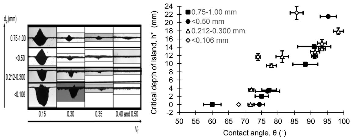
Figure 4: Critical island depth,  $h^*$ , formed by silanised glass beads of different  $d_p$  at different  $V_f$  (left). Effect of the bead contact angle and particle size on the critical island depth,  $h^*$  (right).
