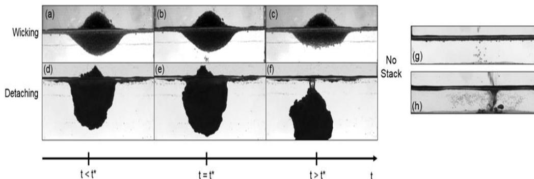
Figure 5: Images of islands at  $V_f=0.15$ , (a)-(c) experienced wicking (for  $d_p=0.75-1.00$  mm), (d)-(f) experienced detaching from the interface (for  $d_p = 0.212-0.300$  mm). Images of the system that can only support rafts instead of islands at  $V_f \geq 0.40$ .  $d_p = 0.75 - 1.00$  mm (g) and  $d_p = 0.212-0.300$  mm (h).
