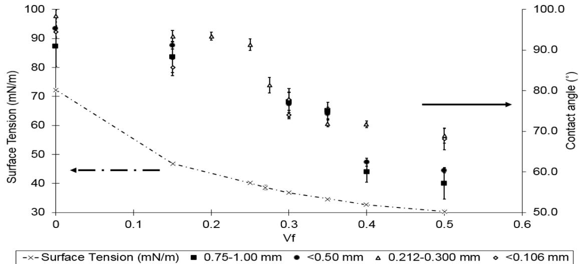
Figure 3: Contact angle of silanised glass beads of different diameter,  $d_p$  as a function of the liquid ethanol volume fraction,  $V_f$ . The crosses refer to the surface tension as a function of  $V_f$ .
