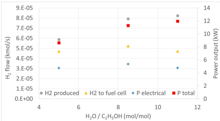
Figure 3: H<sub>2</sub> productivity and H<sub>2</sub> fed to the fuel cell; electrical and total power output as a function of the water/ethanol ratio in the feed. Catalyst mass 3 kg, reformer average temperature 635 °C.
