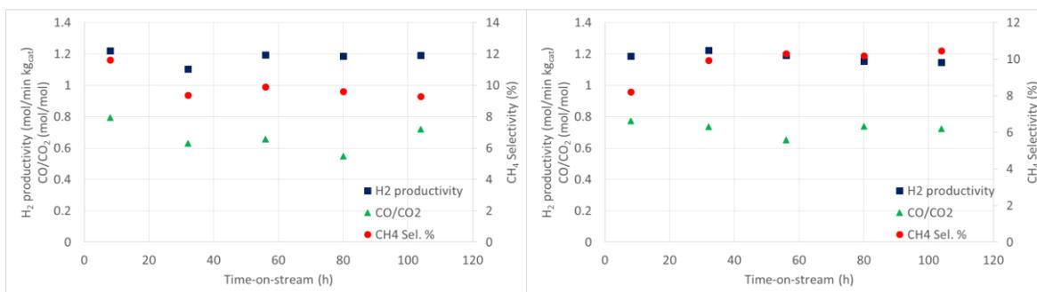
Figure 5: Ethanol steam reforming tests (5 days) using a) BE50, b) BE90.  $T = 500^{\circ}\text{C}$ ,  $W/E = 3: 1 \text{ mol/mol}$ ,  $GHSV = 2,500 \text{ h}^{-1}$ . Each point represents the average of at least 10 samplings (one each hour) every day.
