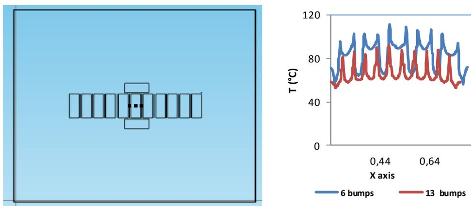
Figure 7: Temperature result differences between 6 and 13 bumps simulations
