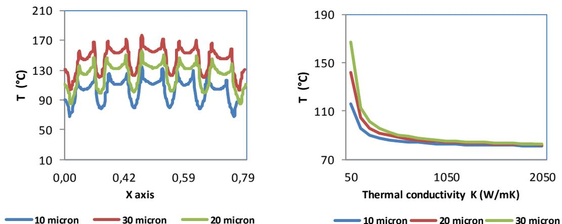
Figure 4: Temperature profile along x axis gained at different bumps heights and with  $K=60$  W/mk. Temperature profile Vs thermal conductivity at the device centre for different bumps' connection height.
