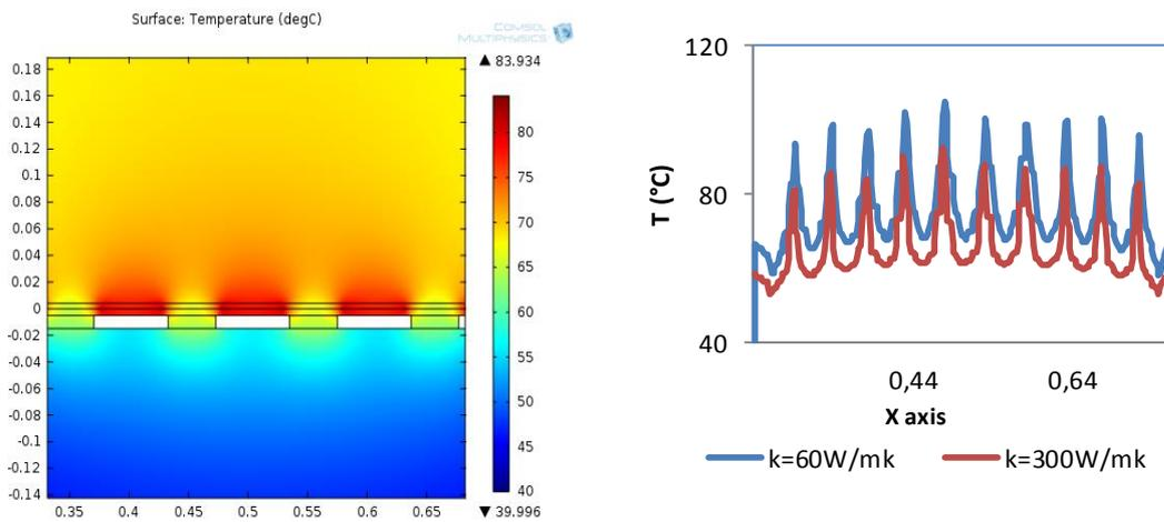
Figure 6: Left side: device Temperature with bumps' connection height of 10  $\mu\text{m}$  and with Au layer  $K_{\text{bumps}}=300\text{ W/mk}$ . Right side: Temperature profile along x coordinate (bumps height of 10  $\mu\text{m}$ ).
