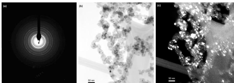
Figure 8 - (a) diffraction pattern. (b) bright field image. (c) dark field image focused on a sample of TiN synthesized 1173K.
