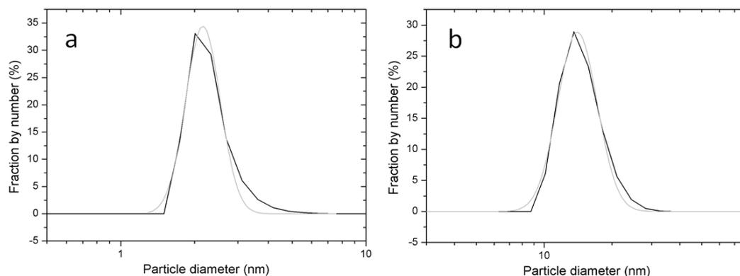
Figure 1: Populations of particle diameters obtained by DLS (black lines) with respective log-normal best fitting curves (gray lines). (a): sample obtained using pure TEA; average diameter=2.2 nm. (b): sample obtained using 50-50% TEA-PG; average diameter=14.6 nm.
