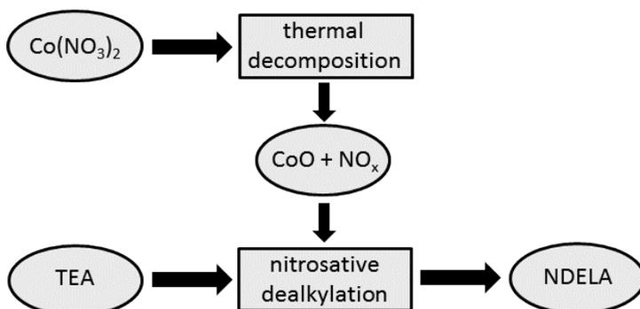
Figure 2: Scheme of a possible sequence of reactions for the synthesis of NDELA from TEA.
