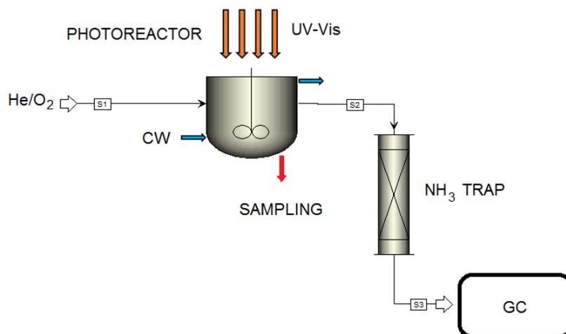
Figure 1: Sketch of the photoreactor used. CW = cooling water.
