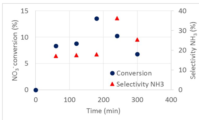
Figure 4: Nitrate conversion and selectivity to NH<sub>3</sub> versus time. Catalyst composition: 0.1 wt% Pd/TiO<sub>2</sub> prepared by FP.
