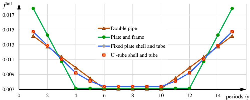
Figure 1: Failure rates of different types of HEs
