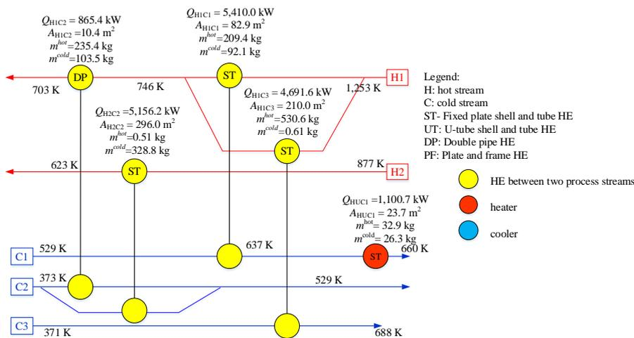
Figure 4: HEN design when the average safety limit is set to average risk limit of design in Figure 3
