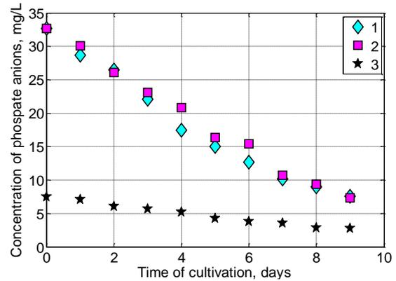
Figure 5: Kinetics of the changes in phosphate anions concentration in wastewater during the cultivation of *C. vulgaris* Beijer IPPAS C-2
