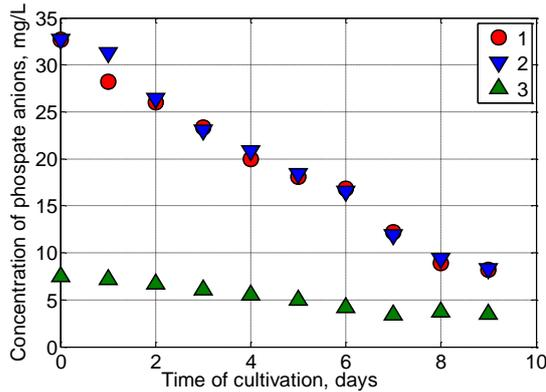
Figure 4: Kinetics of the changes in phosphate anions concentration in wastewater during the cultivation of *C. vulgaris* IFR C-111
