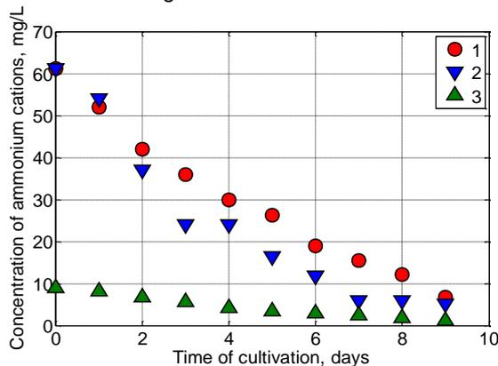
Figure 6: Kinetics of the changes in ammonium cations concentration in wastewater during the cultivation of *C. vulgaris* IFR C-111
