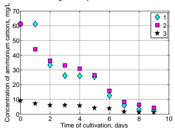
Figure 7: Kinetics of the changes in ammonium cations concentration in wastewater during the cultivation of *C. vulgaris* Beijer IPPAS C-2
