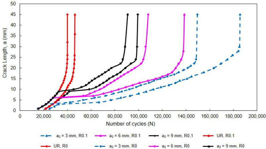
Figure 4: Initial crack length effect on fatigue life for stress ratios  $R0$  and  $R0.1$
