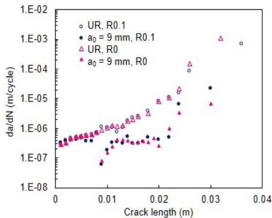
Figure 7: FCGR of unrepaired and repaired for  $a_0 = 9$  mm specimen
