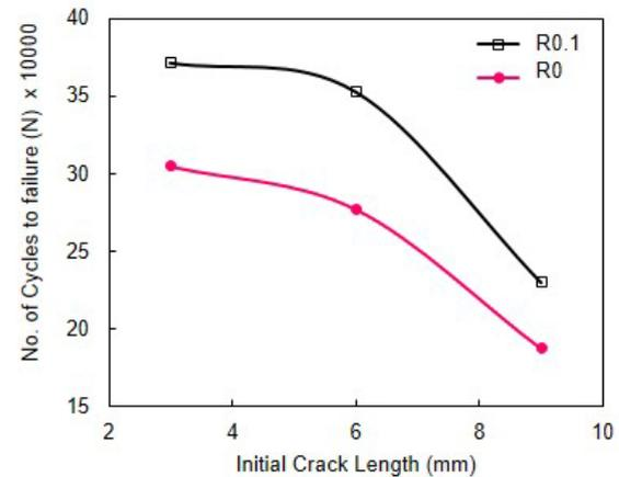
Figure 8: Initial crack length effects on the fatigue life of patched crack plates loaded at two stress ratios
