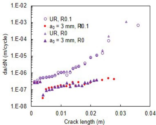
Figure 5: FCGR of unrepaired and repaired for  $a_0 = 3$  mm specimen
