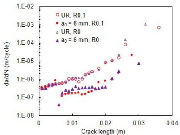
Figure 6: FCGR of unrepaired and repaired for  $a_0 = 6$  mm specimen
