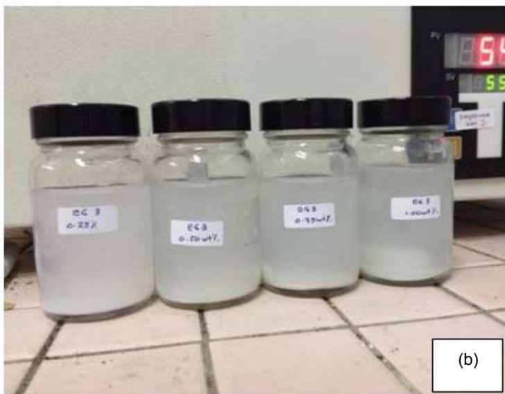
Figure 2: Nanofluids with surfactant: (a) Upon preparation with surfactant; (b) After 2 weeks with surfactant Thermal
