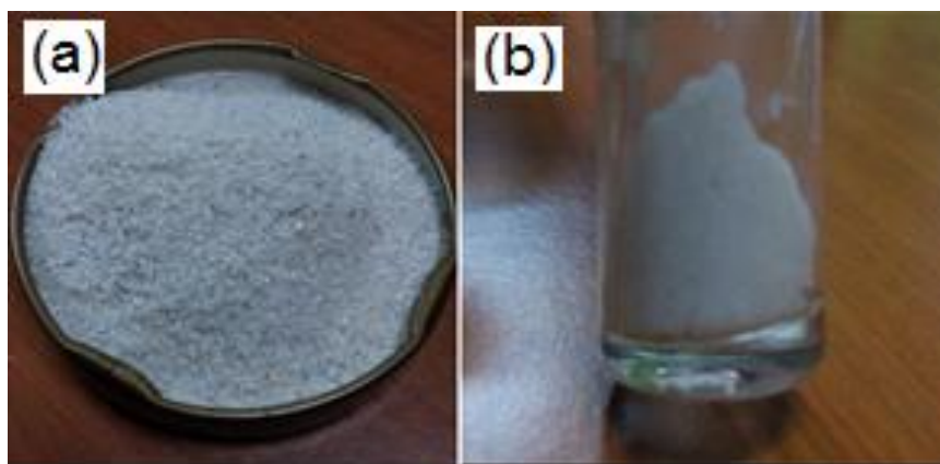
Figure 1: Photograph images of a) dried bacterial cellulose and b) BCNW after acid hydrolysis
