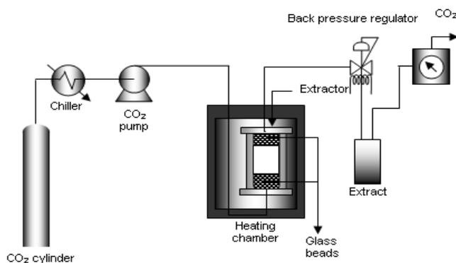
Figure 2: Schematic diagram of supercritical CO<sub>2</sub> extraction apparatus
