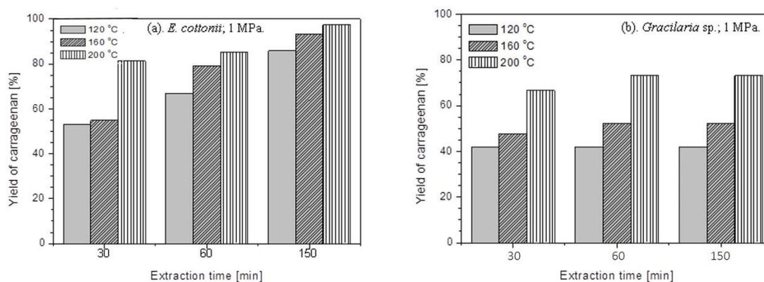
Figure 4: Yield of extracted carrageenan at constant pressure of 1 MPa and various extraction temperatures
