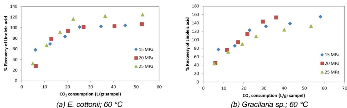
Figure 7: Recovery of Linoleic acid extracted by supercritical  $\text{CO}_2$  at constant temperature of 60 °C and various extraction pressures
