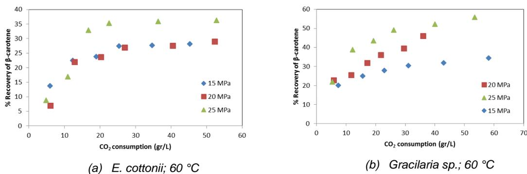
Figure 6: Recovery of  $\beta$ -carotene extracted by supercritical  $\text{CO}_2$  at constant temperature of 60 °C and various extraction pressures
