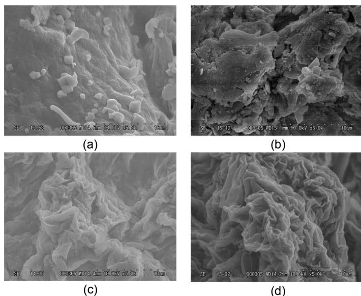
Figure 3: SEM images of (a) starting material of *E. cottonii*, (b) starting material of *Gracilaria sp.*, (c) residue of *E. cottonii*, and (d) residue of *Gracilaria sp.*
