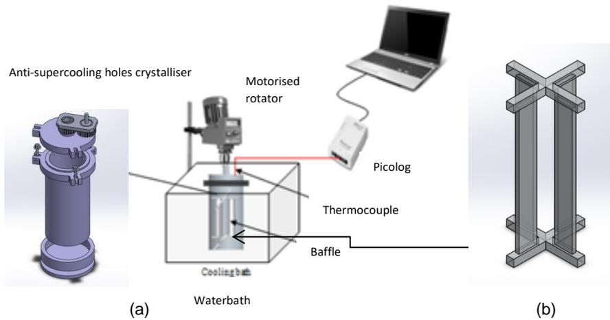
Figure 1: (a) Schematic diagram for experimental setup (b) Illustration of baffle
