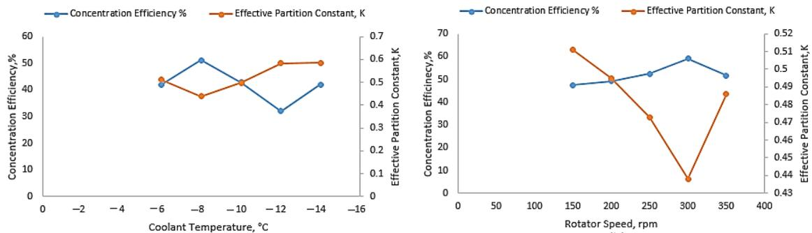
Figure 2: (a) Effect of coolant temperature on  $K$ -Value and concentration efficiency (b) Effect of rotator speed on
