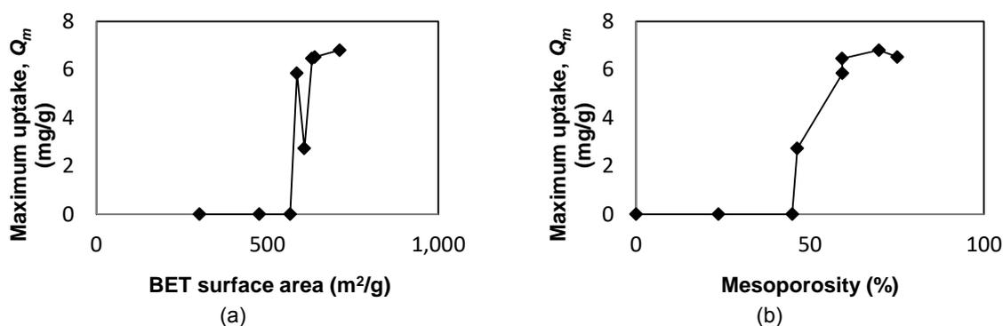
Figure 2: Possible influenced properties on adsorption of RO16: (a) BET surface area and (b) mesoporosity
