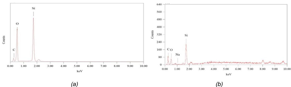
Figure 4: EDS results of (a) raw and (b) treated rice husk
