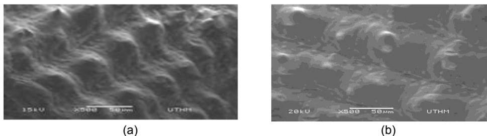
Figure 3: SEM micrograph of (a) raw, (b) treated rice husk
