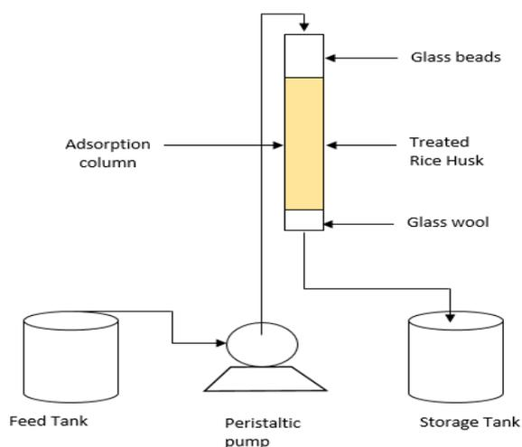
Figure 1: The cadmium adsorption set-up
