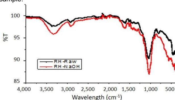
Figure 2: FTIR spectra of the raw and NaOH treated rice husk
