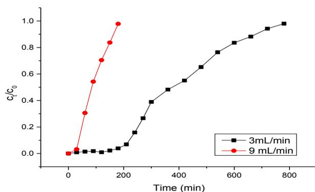
Figure 6: Effect of cadmium solution flow rate at constant bed height of 2.8 cm and 5 mg/L concentration
