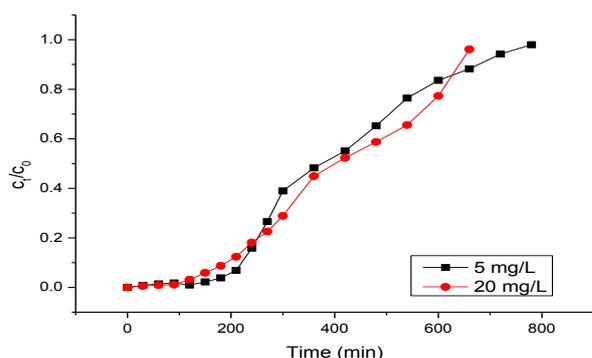
Figure 5: Effect of cadmium concentration at fixed bed height of 2.8 cm and flow rate of 3 mL/min
