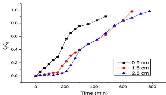
Figure 7: Effect of bed heights at 5 mg/L concentration and flow rate of 3 mL/min
