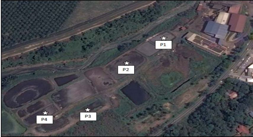
Figure 1: Odor sampling at the palm oil mill effluent treatment ponds specifically at the acid pond (P1), anaerobic pond (P2), facultative pond (P3) and aerobic pond (P4)
