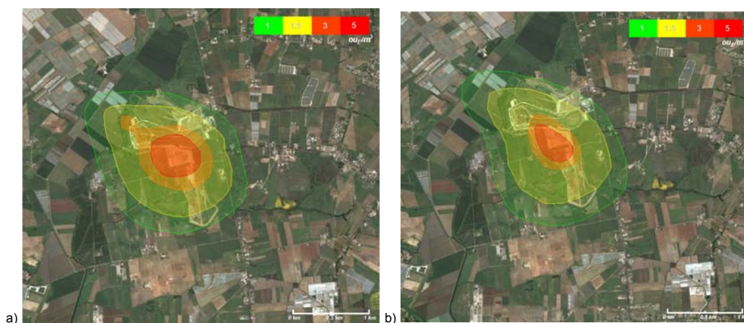
Figure 3: Maps of the 98 th percentile of the hourly peak odour concentration – a) Current scenario; b) Project scenario
