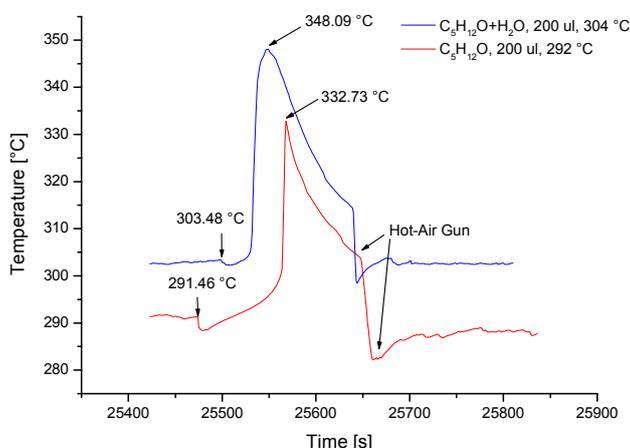
Figure 8: Comparison of two individual AIT test results of 1-pentanol with and without water at the same experimental conditions
