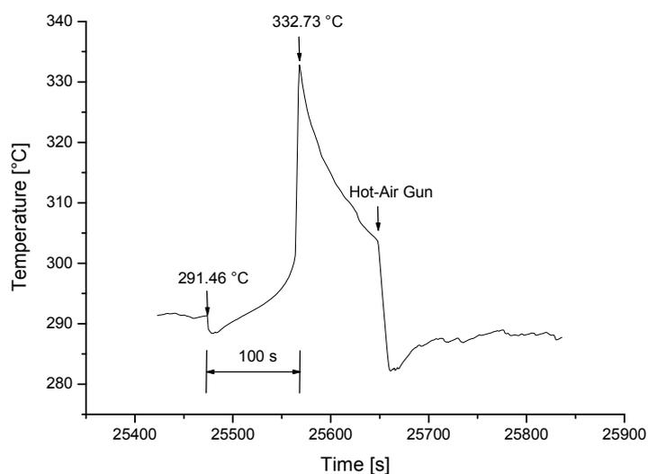
Figure 5: Time history of a typical autoignition experiment ( $C_5H_{12}O$ , 200  $\mu$ l, 292  $^{\circ}$ C)
