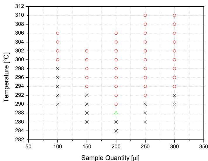
Figure 6: Ignition temperature at different sample volumes for 1-pentanol (circle: flammable case; cross: non-flammable case; triangle: the lowest flammable temperature)
