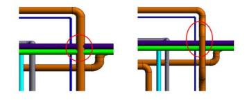
Figure 2: Pipeline collision schematic diagram
