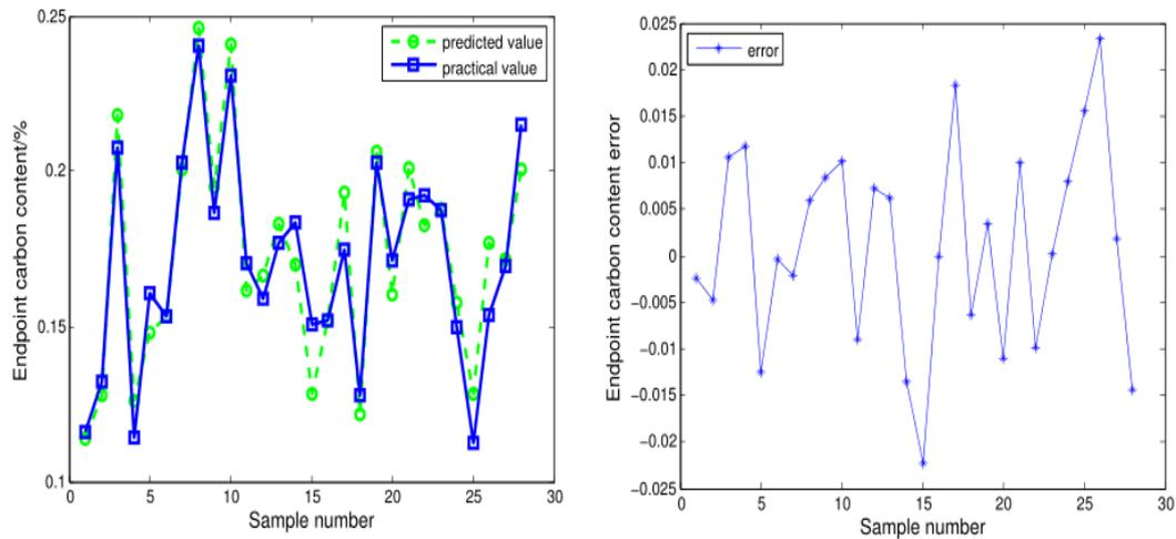
Figure 2: Prediction of endpoint carbon content
