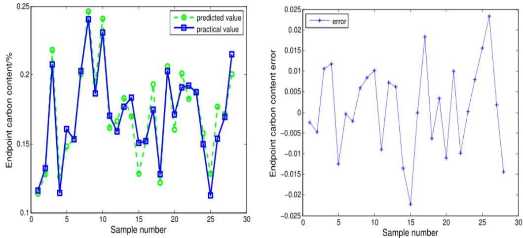
Figure 2: Prediction of endpoint carbon content
