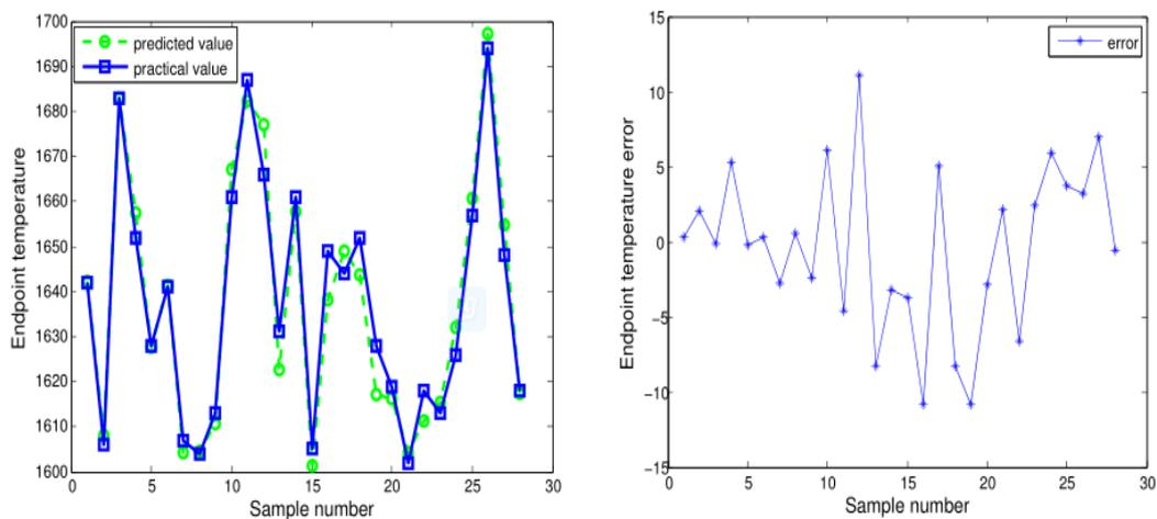
Figure 3: Prediction of endpoint temperature
