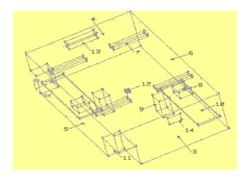
Figure 2: The mixed ventilation air conditioning system model in the office (Side to side back to type)
