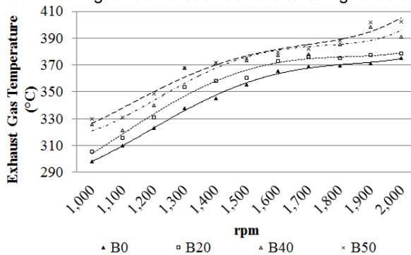
Figure 5: Variation in EGT with engine speed
