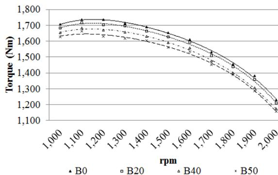
Figure 2: Variation in torque with engine speed
