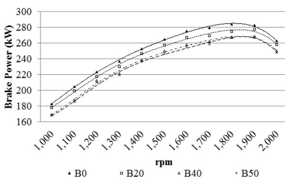
Figure 1: Variation in BP with engine speed
