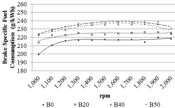
Figure 3: Variation in BSFC with engine speed
