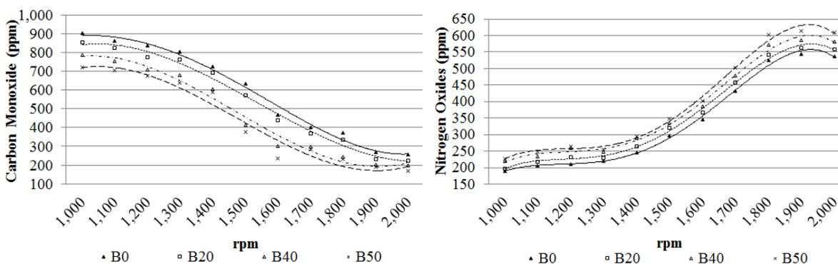
Figure 7: Variation in CO emissions with engine speed Figure 8: Variation in NOx emission with engine speed
