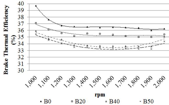
Figure 4: Variation in BTE with engine speed
