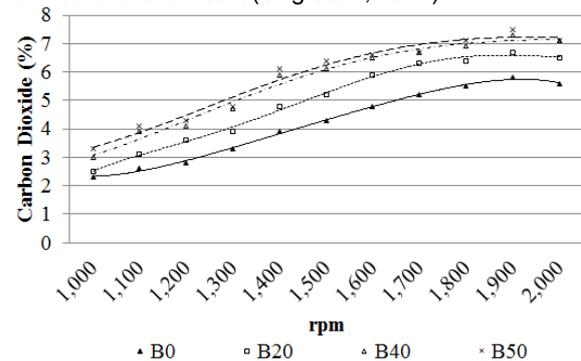
Figure 6: Variation in CO<sub>2</sub> emissions with engine speed
