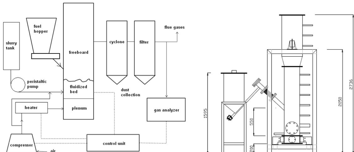
Figure 1: Schematics of the fluidized bed facility for pilot combustion tests.
