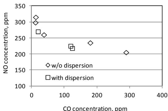
Figure 4: NO versus CO concentration in the flue gas.
