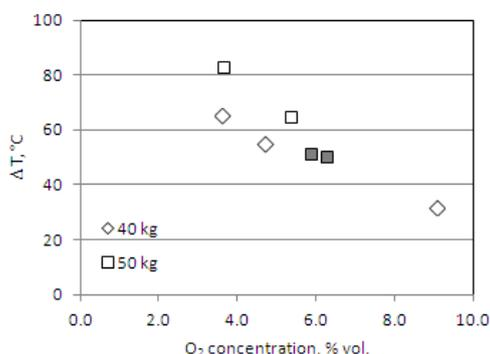
Figure 3: Temperature increase in the freeboard versus  $O_2$  concentration in the flue gas for two different bed inventories.
