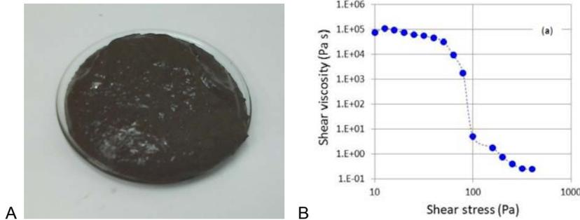
Figure 2: photograph of LS/RS/H<sub>2</sub>O slurry (A) and viscosity of the slurry versus shear rate at 25 °C (B).
