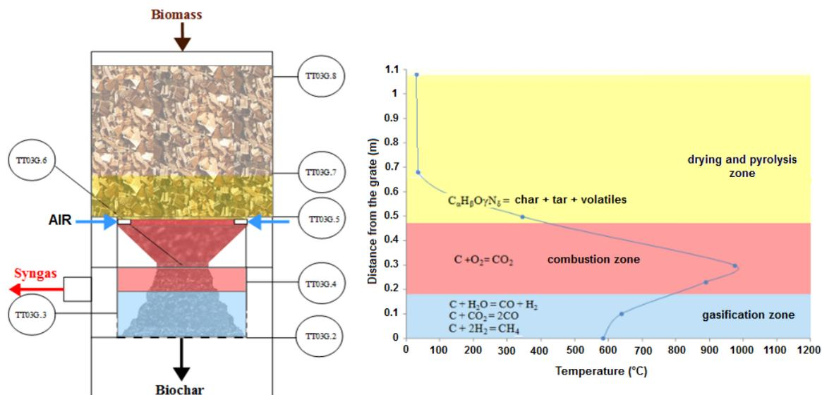
Figure 2: Average temperature profile at the stationary state along the gasifier at ER = 0.3
