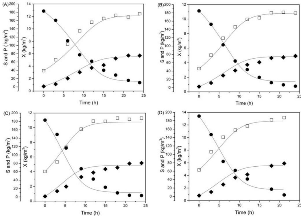
Figure 1: Experimental measures (substrate (●), cell (□) and ethanol (◆)) compared with the performance of the model (—) at: (A) 30 °C; (B) 32 °C; (C) 34 °C and (D) 36 °C.
