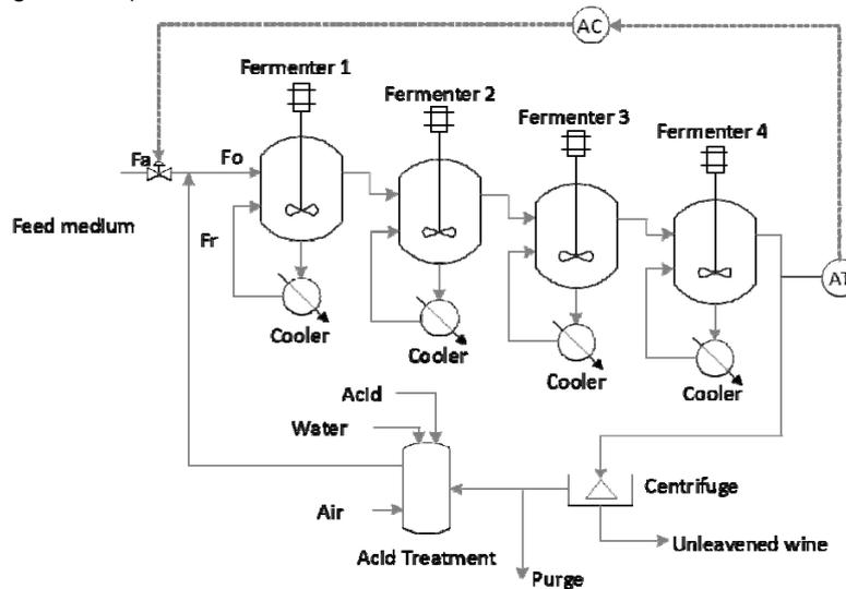
Figure 2: General scheme of the continuous fermentation process
