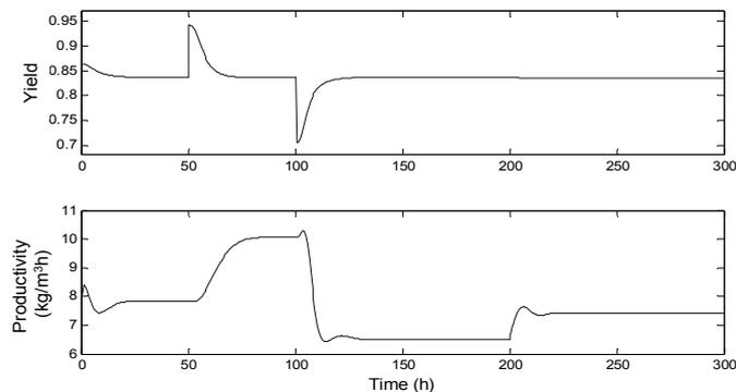
Figure 4: Yield and Productivity ( $\text{kg/m}^3\text{h}$ ) responses of the simulation for the fermentation process in closed-loop.
