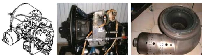
Figure 7: Garret microgas turbine: main scheme (left), view of the system (center) and silo-type combustion chamber (right).
