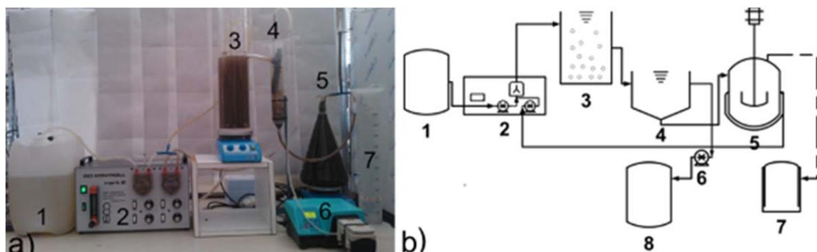
Figure 1: a) Experimental set-up, b) PFD: 1) Influent barrel, 2) Control system, 3) Oxidation reactor, 4) Settling tank, 5) Anaerobic sludge holding tank, 6) Peristaltic pump, 7) Gasometer, 8) Effluent barrel
