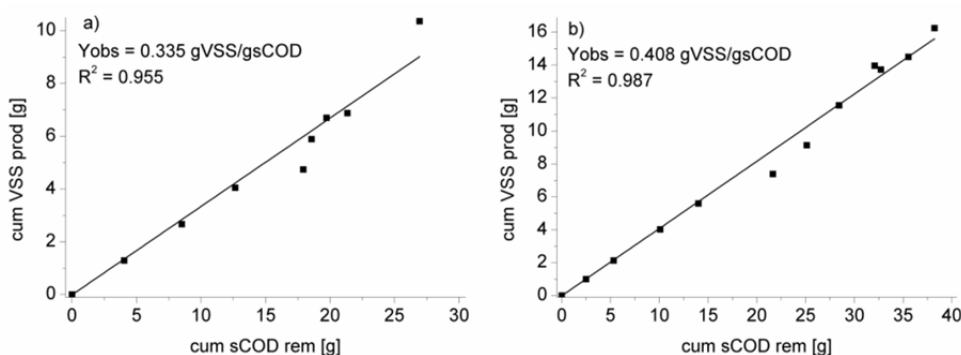
Figure 3: Observed yield from cumulative biomass production and organic matter removal: a) run #1, b) run #2
