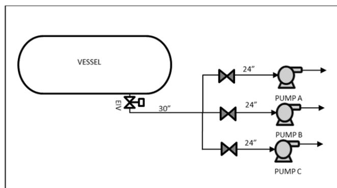
Figure 3: Multiple pumps with large volume in suction
