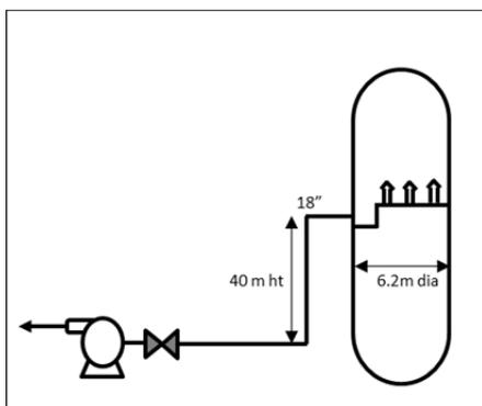
Figure 2: Pump drawing suction from chimney tray
