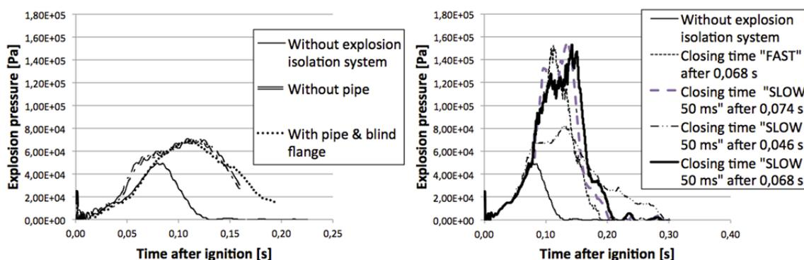
Figure 4: Pressure/time courses of the numerical tests
