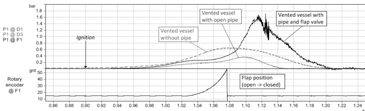
Figure 2: Exemplary pressure/time-curves of the registered reduced explosion overpressures inside the test vessel (test series 1, tests D1, D3, F1)
