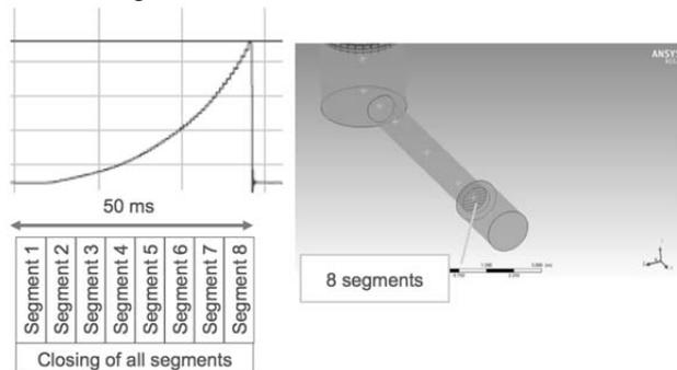
Figure 3: Modelling of the closing phase of an explosion isolation flap valve
