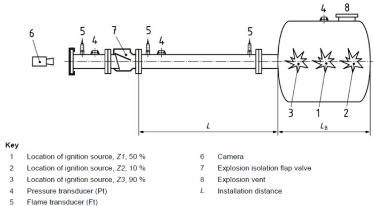
Figure 1: Test condition for the functionality test - module C of EN 16447
