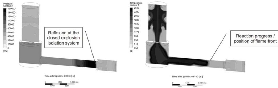
Figure 5: Pressure and temperature courses immediately after the closing of the explosion isolation – calculation model „FAST after 0,068 s“
