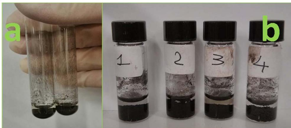
Figure 1 a) hydrogel floating in water; b) swelling effect of acid and basic media on the network
