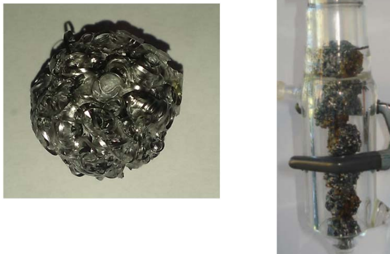
Figure 1: Spherical wads of stainless-steel fibre with dried gelatinized starch.
