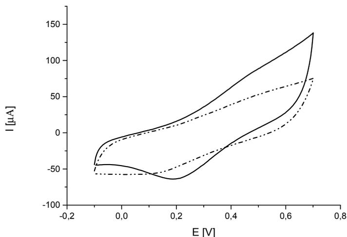
Figure 3: Electrode responses recorded in 0.2 mM catechol, pH 5.2; solid line – Pt electrode modified with polymer and laccase, dotted line – Pt electrode modified with polymer. Measurement conditions: scan rate  $100 \text{ mV s}^{-1}$ , Ag/AgCl – reference electrode.
