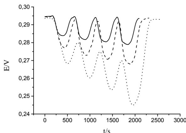
Figure 4: The output signal of the produced biosensor for different flow rates: 150  $\mu\text{l}/\text{min}$  – solid line, 75  $\mu\text{l}/\text{min}$  – dashed line and 25  $\mu\text{l}/\text{min}$  – dotted line
