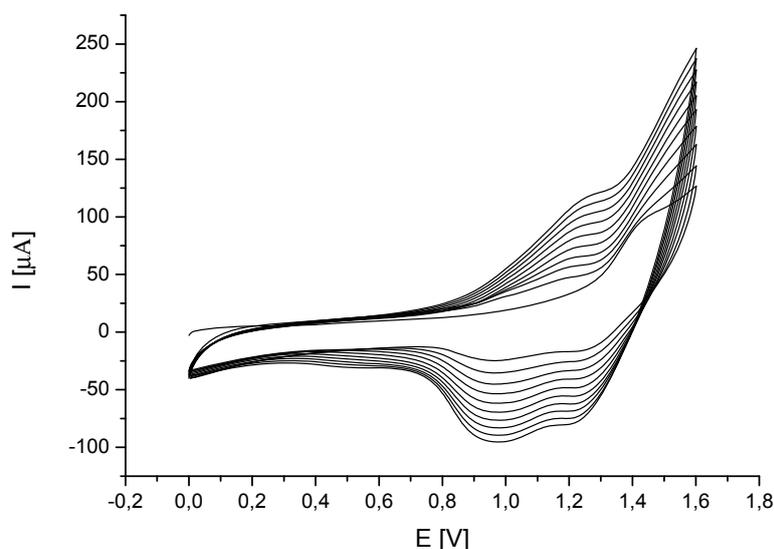
Figure 2: Cyclic voltammograms of investigated monomer; (2,7-bis(carbazole)-N-hexylacridone - 1mM) in 0.1 M TBA-TFB. Measurement conditions: scan rate  $50 \text{ mV s}^{-1}$ , Ag/AgCl – reference electrode, 10 cycles.
