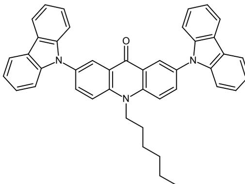
Figure 1: Structure of monomer - 2,7-bis(carbazole)-N-hexylacridone.
