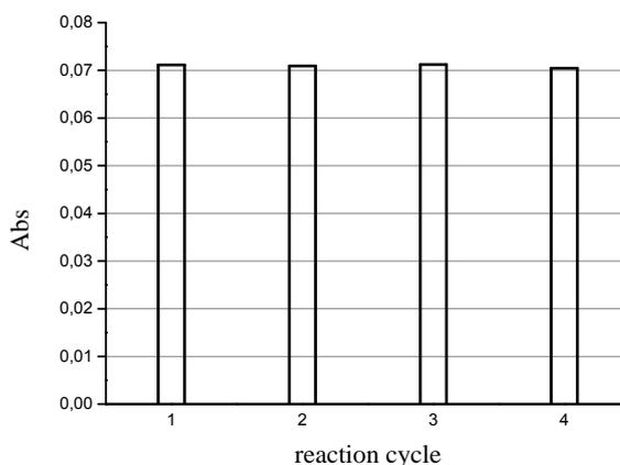
Figure 4: Absorbance recorded in consecutive measuring cycles, measurement conditions: flow rate – 50  $\mu\text{l}/\text{min}$ , LED current: 15 mA, ABTS concentration: 180  $\mu\text{M}$
