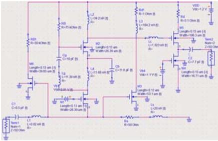
Figure 3: Schematic of the proposed LNA
