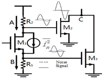
Figure 2: Principle of noise cancelling technique
