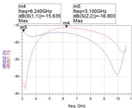
Figure 5: Simulated  $S_{11}$  and  $S_{22}$  against frequency characteristics of 3.1-10.6 GHz UWB LNA
