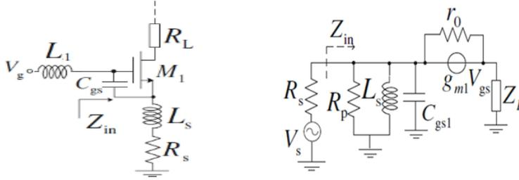
a The Proposed IMN Topology      b The equivalent small signal model of the circuit in Fig. 2a
