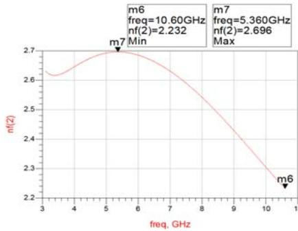
Figure 6: Simulated NF against frequency characteristics of 3.1-10.6 GHz UWB LNA
