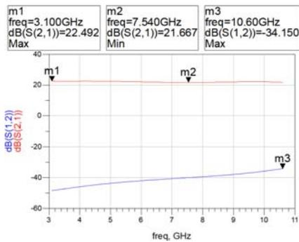
Figure 4: Simulated  $S_{21}$  and  $S_{12}$  against frequency characteristics of 3.1-10.6 GHz UWB LNA
