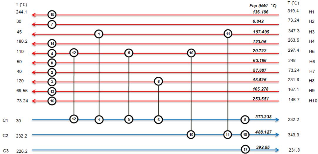
Figure 3: The Grid Diagram of the original HEN from Siemanond and Kosol (2012)
