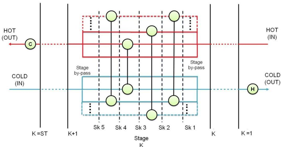
Figure 1: The grid diagram (Linnhoff and Hindmarsh, 1983) representing modified and extended stage-wise superstructure of Yee and Grossmann (1990) with non-isothermal mixing allowing several exchanger matches per branch stream
