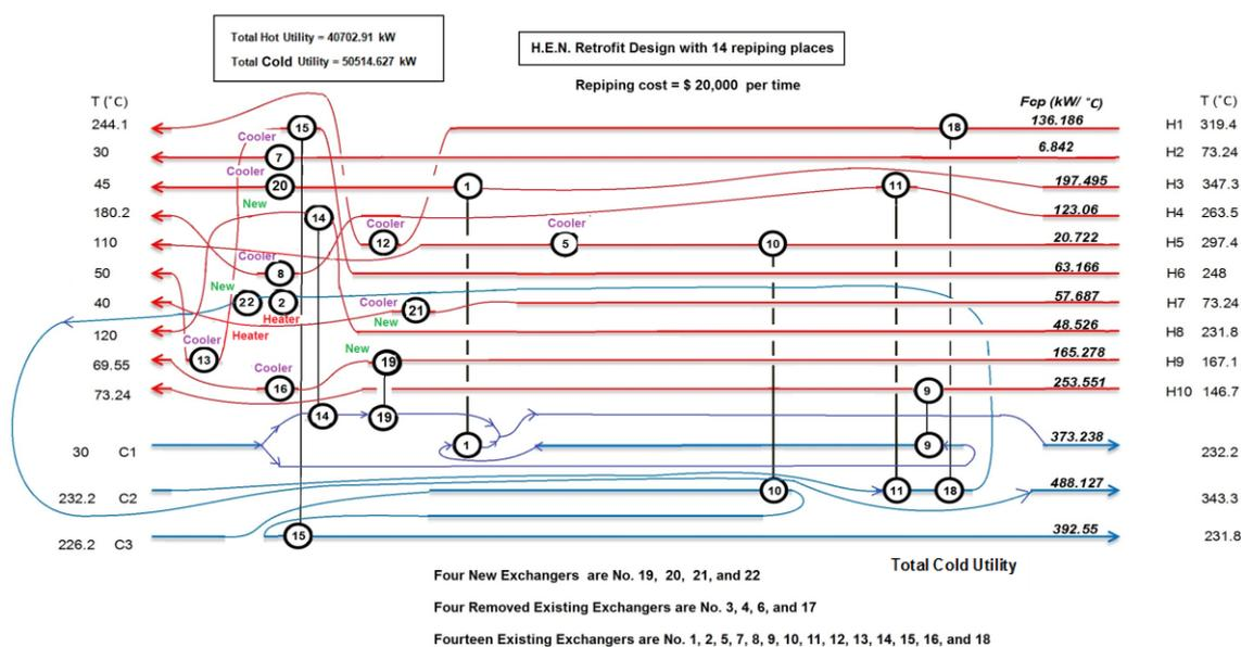
Figure 5: The Grid diagram of retrofit case from our work with repiping representation
